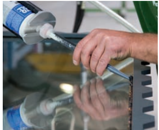
Applying the 2C silicone for wood-glass composite elements
